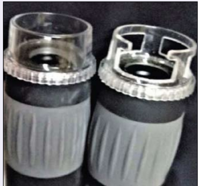
Fig 1. The terminal ends of 2 identical universal serial bus (USB) video dermatoscopes (E-scope video dermatoscope, Timpac Healthcare Pvt Ltd, New Delhi, India). The USB video dermatoscope on the left shows the original acrylic rim. The video dermatoscope on the right has been simply engineered by cutting out polygonal windows in the rim
