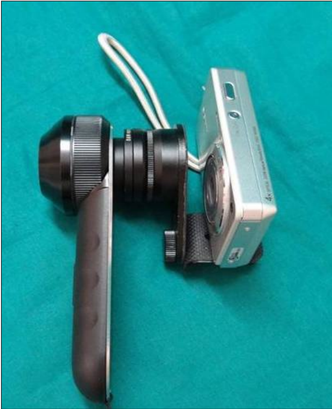
Figure 3: Dermoscopy is attached to a dedicated camera to save the captured images. This adapter makes dermoscope to fit correctly only to recommended model by the company.
