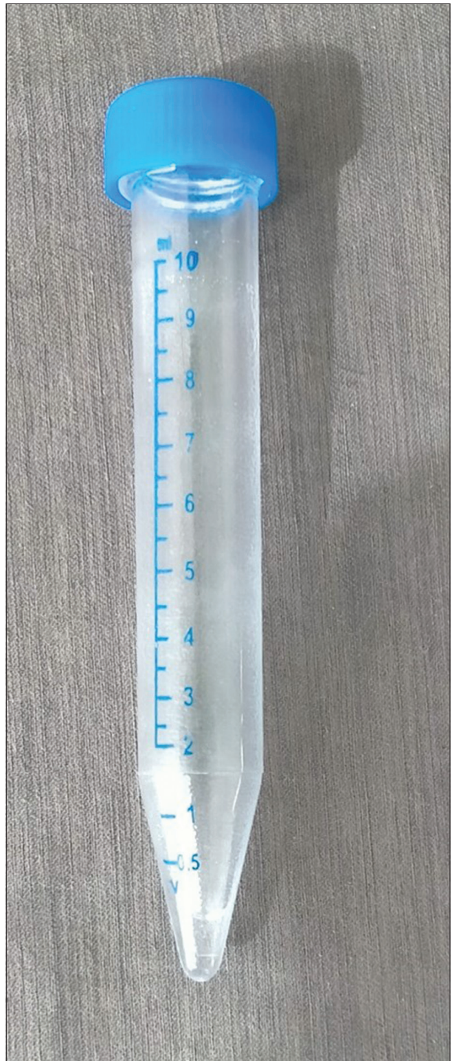
Figure 2: Shows a screw top plastic tube which needs to be individually sterilized using ethylene oxide (ETO)
