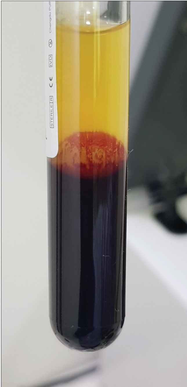
Figure 8: Shows smearing of cells on the back wall of the tube in a fixed-angle centrifuge
